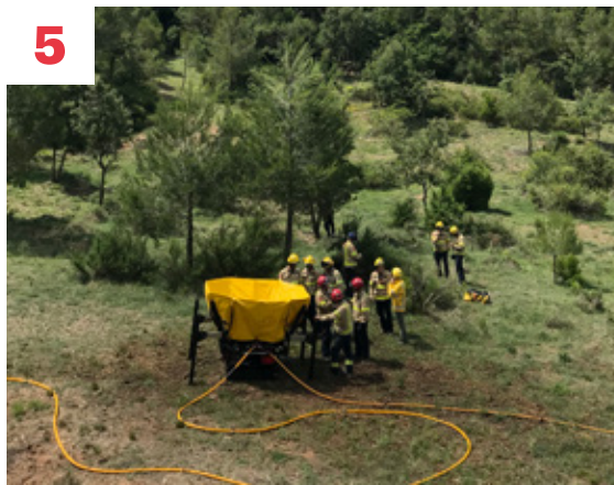
5 Tank assembly A light structure for easy water tank deployment and assembly. Tank connection to the pump via a suction hose.
