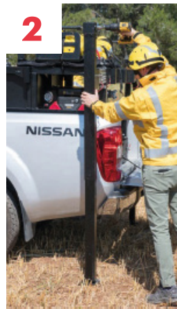
2 Loading and unloading Telescopic legs to raise the Heliskid to load/unload it from the vehicle.
