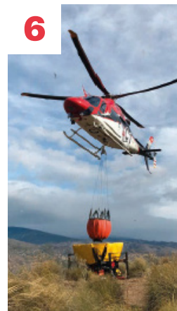
6 Filling The tank can be filled from the helicopter or through suction from a hydrant, river, lake, truck, etc.
