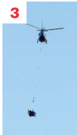
3 Helitransportable Because of the weight (350 kg) and 4 upper anchoring points, the Heliskid may be transported to difficult-to-access areas via helicopter.
